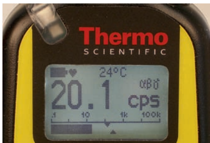
Simultaneous measurement of alpha-, beta-, and gamma radiation
